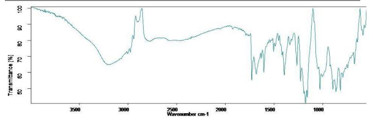
Fig 4. FTIR spectrum of Drug + Di-Calcium Phosphate.
