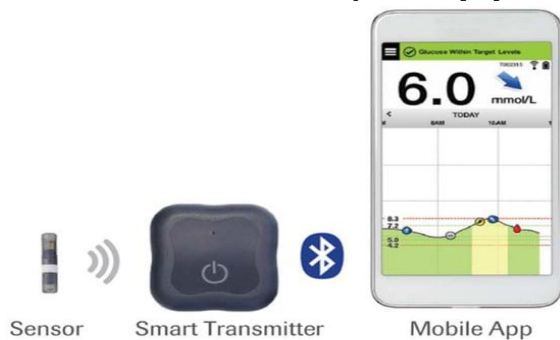
Figure 3. Example of Implantable CGM System Based on optical sensing technique, the Senseonics everSense continuous glucose monitoring system.
